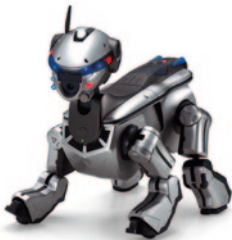
↑ ERS-220, 2001. This AIBO has a more futuristic sci-fi aesthetic. A set of LEDs express emotions: blue when it is happy and red if it is angry.
