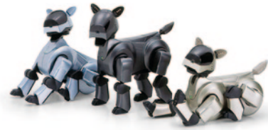
↑ ERS-210, 2000. The second-generation AIBO. With an increase in the number of sensors and LEDs, it is more expressive of emotions such as joy. It also has voice recognition functions and the ability to take photos.
