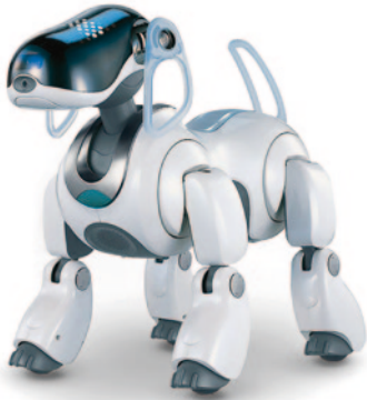
↑ ERS-7, 2003. This version of AIBO can connect wirelessly with other electronic devices and show a wide range of emotions through its lively LED-illuminated face. Masaya Matsuura, a musician and video game designer, composed sounds for this model.
